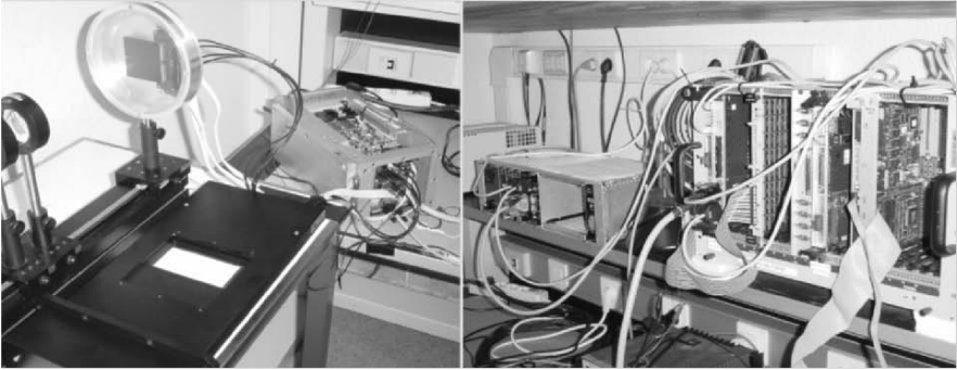
Figure 1. (left) OSIRIS DAS including a couple of eng-E2V44.82 CCDs in the test bench. (right) Main control crate.
