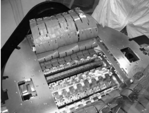
Figure 4. Flex circuits inside the cryostat. In this figure one of the outer rows of CCDs is already installed and connected. Zener diodes are soldered onto the flex circuit to provide ESD protection.
