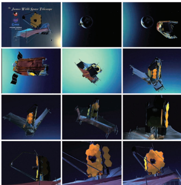
Figure 7. JWST deployment. The time sequence is from left to right and from top to bottom. Deployment steps are as follows: (1) fully deployed observatory showing partner logos, (2) JWST leaving earth following Ariane V launch, (3) beginning of deployment, (4) solar panels deploy, (5-8) sunshade deploys, (9) mast deployment, (10) secondary mirror deployment, and (11-12) primary mirror deployment. For scale, the primary mirror is about 6.5-meters in diameter and the sunshade is about the size of a tennis court.
