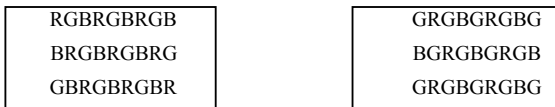
Figure 1. Two types of Bayer filters: the letters R,G and B (Red, Green and Blue) filtered pixels. The left matrix has a perfect balance of R, G and B pixels. The right one, which is used mainly for photography and TV applications, has 50% of the pixels filtered in green to increase the luminosity information of the images.
