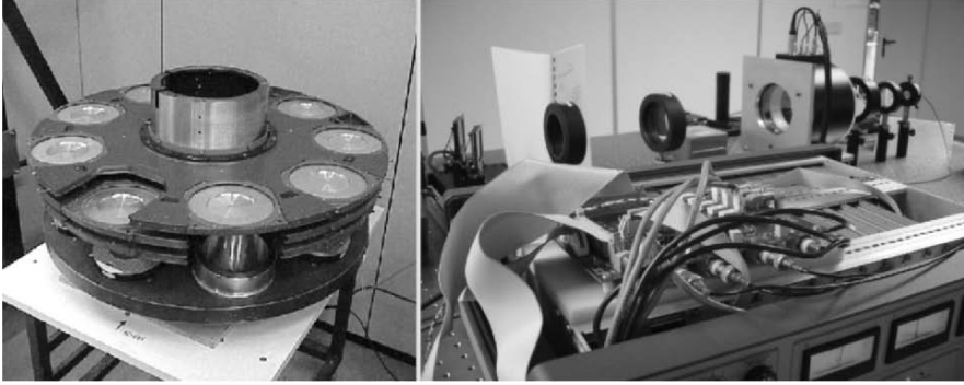
Figure 3. (left) Filter wheels. They include pupil masks, conventional filters and light dispersive elements (grisms). (right) Main elements mounted in the last wheel are the two tunable filters, which convert OSIRIS into a very versatile instrument. Development of the four wheels has been carried out by NTE (Barcelona, Spain). Tunable filters are made by ICOS (London, UK), with a new entire FPGA-based control developed by the OSIRIS team (see Gigante, et al. [3]).
