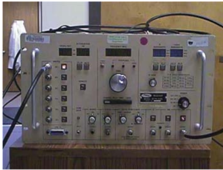
Fig. 15.7 A second-hand wideband, wide-bandwidth receiver.
