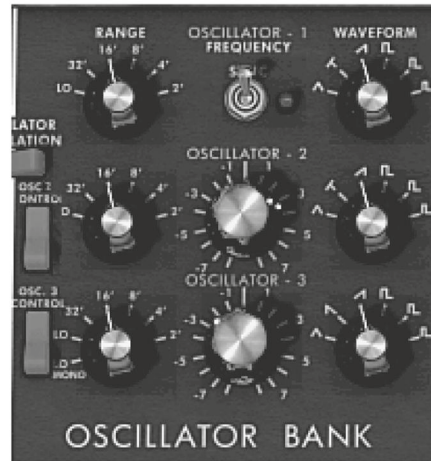
A creative use of the beating is a thickening of a sound by using two oscillators set to pitches separated by less than 50 cents, as seen above on the Arturia Minimoog. In this example Oscillator-2 is shifted up by about 2% and Oscillator-3 is shifted down by about 5%.
