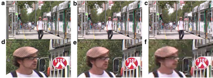
Fig. 3.2 Illustration of inter-view masking effect and depth perception loss in stereoscopic 3-D viewing due to coding distortions [64]. From left to right, top row : (a) an H.264/AVC-coded left view image at 10 Mbps (frame 2 of 3-D video sequence 28 of RMIT3DV database [7]), (b) the right view coded at 2 Mbps, (c) the right view coded at 512 kbps; bottom row : (d) a cropped portion of (a), (e) a cropped portion of (b), and (f) a cropped portion of (c). When (a) and (b) displayed for 3-D viewing, coding distortions in (b) were masked by (a), while (a) and (c) were displayed to the viewer, depth perception was lost due to severe distortions in (c). (Focus your eyes on the center of (b) or (e) image assuming that the point of picture in the real world by the side-by-side visual representation is beyond the screen/page to see stereo 3-D image/frame)
