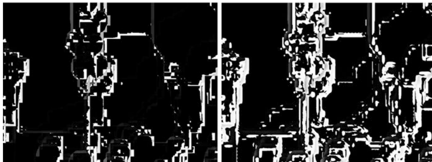
Fig. 6.15 Difference between original depth map and the up-sampled depth map using the nearest-neighbor interpolation ( left ) or bicubic interpolation method ( right ) algorithm for the Balloons sequence. In this case the up-sampling factor is 16 and black pixels indicate no difference [55]
