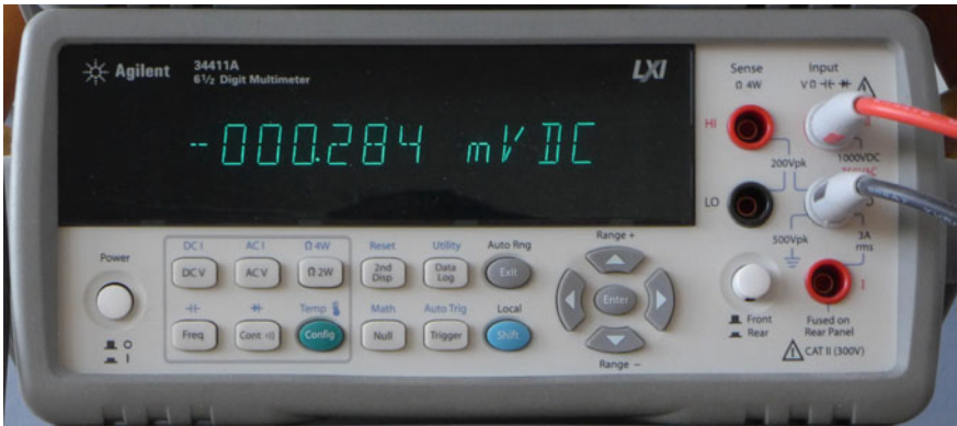
Fig. 3.19 Benchtop multimeter configured for voltage measurements. In order to support four-wire resistance measurements, this instrument has five terminals for connecting the device under test
