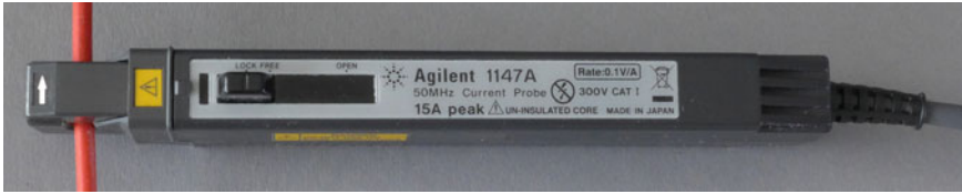
Fig. 3.16 Probe for measuring dynamic currents. The probe picks up and measures the magnetic field produced by the current in the conductor that is threaded through the probe’s core. The arrow indicates the direction of positive currents
