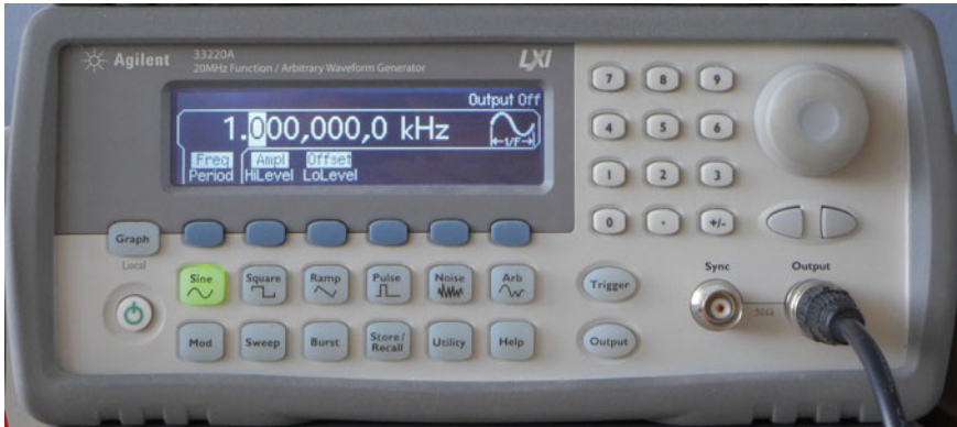
Fig. 2.12 A function generator produces periodic signals within a frequency range from 1\ \mu\text{Hz} up to several megahertz
