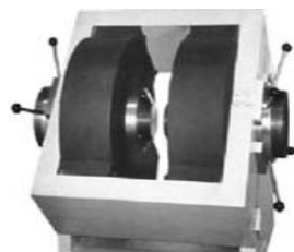
An electromagnet with tapered pole pieces capable of generating 1.8 \text{ MA m}^{-1} .
