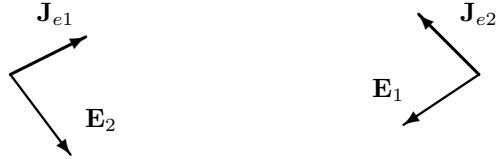
Fig. 6.2 Reciprocity in Gibbsian electromagnetics relates source vectors and their field vectors. For example, if field \mathbf{E}_1 from source \mathbf{J}_{e1} is orthogonal to source \mathbf{J}_{e2} , its field \mathbf{E}_2 is orthogonal to source \mathbf{J}_{e1} provided medium satisfies reciprocity conditions.
