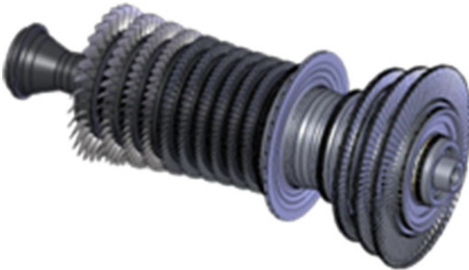
Fig. 7 Gas turbine model
