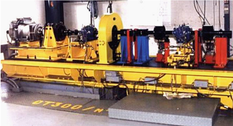
Fig. 11 EUROPE test-rig of Électricité de France (EDF-AMA) equipped with two oil-film bearings and one composed shaft, allowing the insertion of different cracked specimen. Shaft diameter d = 70 mm
