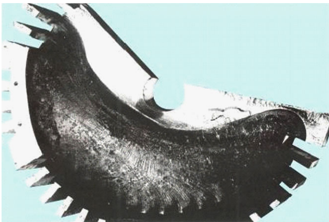
Fig. 4 This crack could be revealed only by means of US inspection from internal hole: photo shows cracked rotor slice (after cutting)
