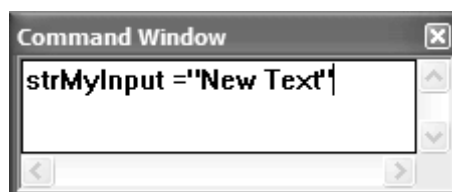
Figure 11.15. The command window also can be used to set the value of variables
