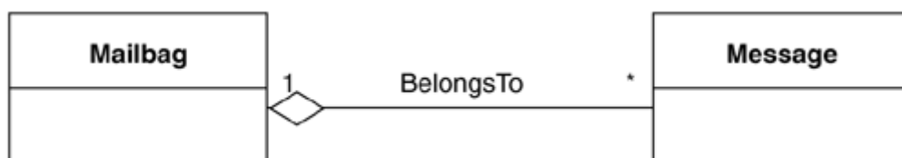
Figure 5.11. Aggregate associations in UML
