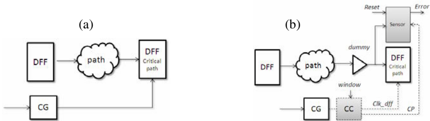
Fig. 6. Critical path before (a) and after (b) the monitoring step. Sensors are added with specific dummy cells allowing an easy place and route. Clock Cells are inserted later.
