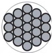
Fig. 2.9 Cross section of 19-strand building wire.
