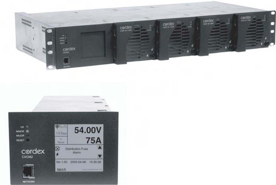
Fig. 3.20 Rectifier shelf assembly with controller and rectifier modules (same type as in Fig. 3.19 but 48 V in this case). The shelf assembly mounts in a standard 19-in. equipment frame. The controller ( bottom photo ) plugs into the left-hand slot of the rectifier shelf assembly and is required for rectifier operation. LED indicators on the upper-left are OK, minor alarm, and major alarm, and there is a reset button just below the LEDs. At the bottom left of the controller is a 10BaseT Ethernet jack for connecting the controller to the central office local area network. The dimensions of the shelf assembly are 17.4 in. wide \times 3.4 in. high \times 12.0 in. deep. (Photos courtesy of Argus Technologies, Inc.)
