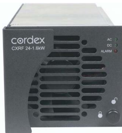
Fig. 3.19 Typical rectifier front panel. The dimensions of this switch-mode rectifier module are 3.94 in. wide \times 3.30 in. high \times 9.25 in. deep and it is rated 1.6 kW at 24 V. The LED indicators on the upper right side of the front panel are ac, dc, and alarm. (Photo courtesy of Argus Technologies, Inc.)
