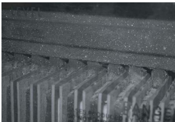
Fig. 6.60 Plate sulfation in shorted cell. (Photo and description courtesy of M.W. Migliaro.)
