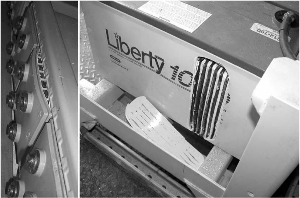
Fig. 6.51 Consequences of excessive plate growth in VRLA cells. (Photos courtesy of M.W. Migliaro.)
