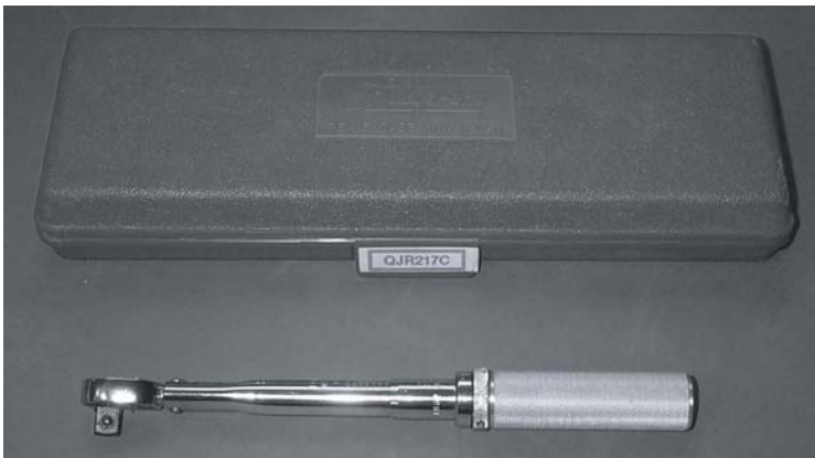
Fig. 6.8 Click-type, micrometer adjustable torque wrench. This wrench is about 12 in. long and has a \frac{3}{8} -in. drive. The torque is set by rotating the handle to the desired micrometer setting.
