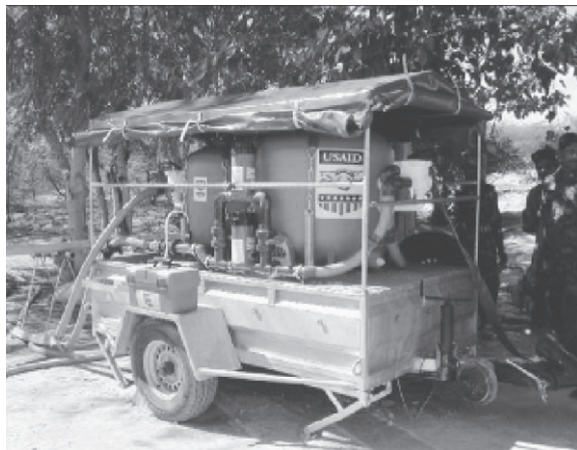
FIGURE 6-3 USAID Office of Foreign Disaster Assistance water purification unit that produced 78,000 liters of water per day for families affected by the January 2001 earthquake in India. (Photo courtesy of Michael Ernst, USAID/OFDA)
