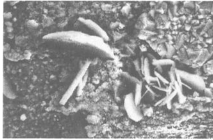
Figure 6 - Secondary electron image showing crystallites composed of Cu, O and S on top of a layer composed of Cu and O on fresh and brown-patinated copper sheet freely for one year in Singapore. (1cm=10µm)
