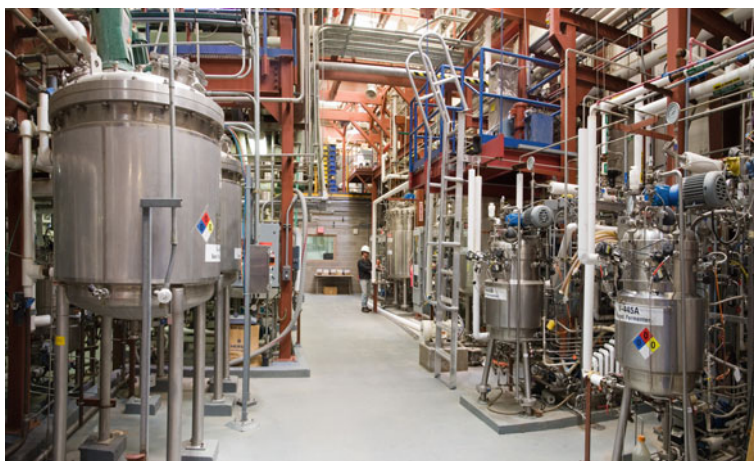
Fig. 6.15 Pilot plant to obtain Ethanol from biomass (this is a photograph from Pat Corkery, Inc/ NREL 16330)
