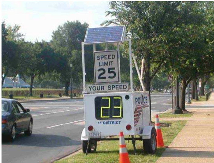
Figure 6.6. Variable message sign displaying the speed limit and the current speed of the vehicles (United States)
