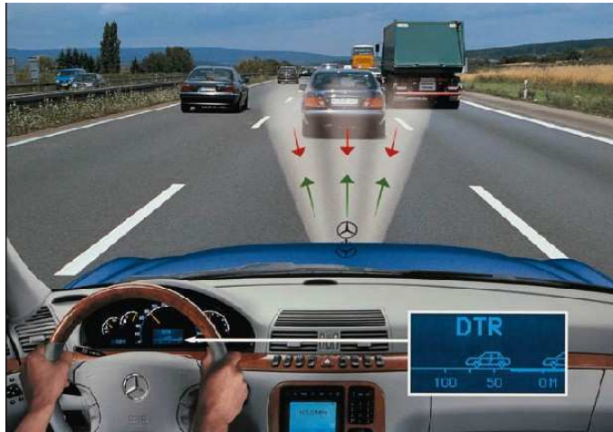
Figure 7.6. Principle of ACC
