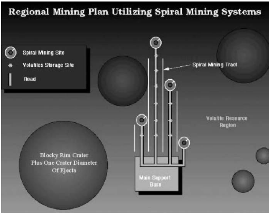
FIGURE 7.3 Regional application of the spiral strategy to production of lunar volatiles. (Courtesy of the University of Wisconsin–Madison Fusion Technology Institute)
