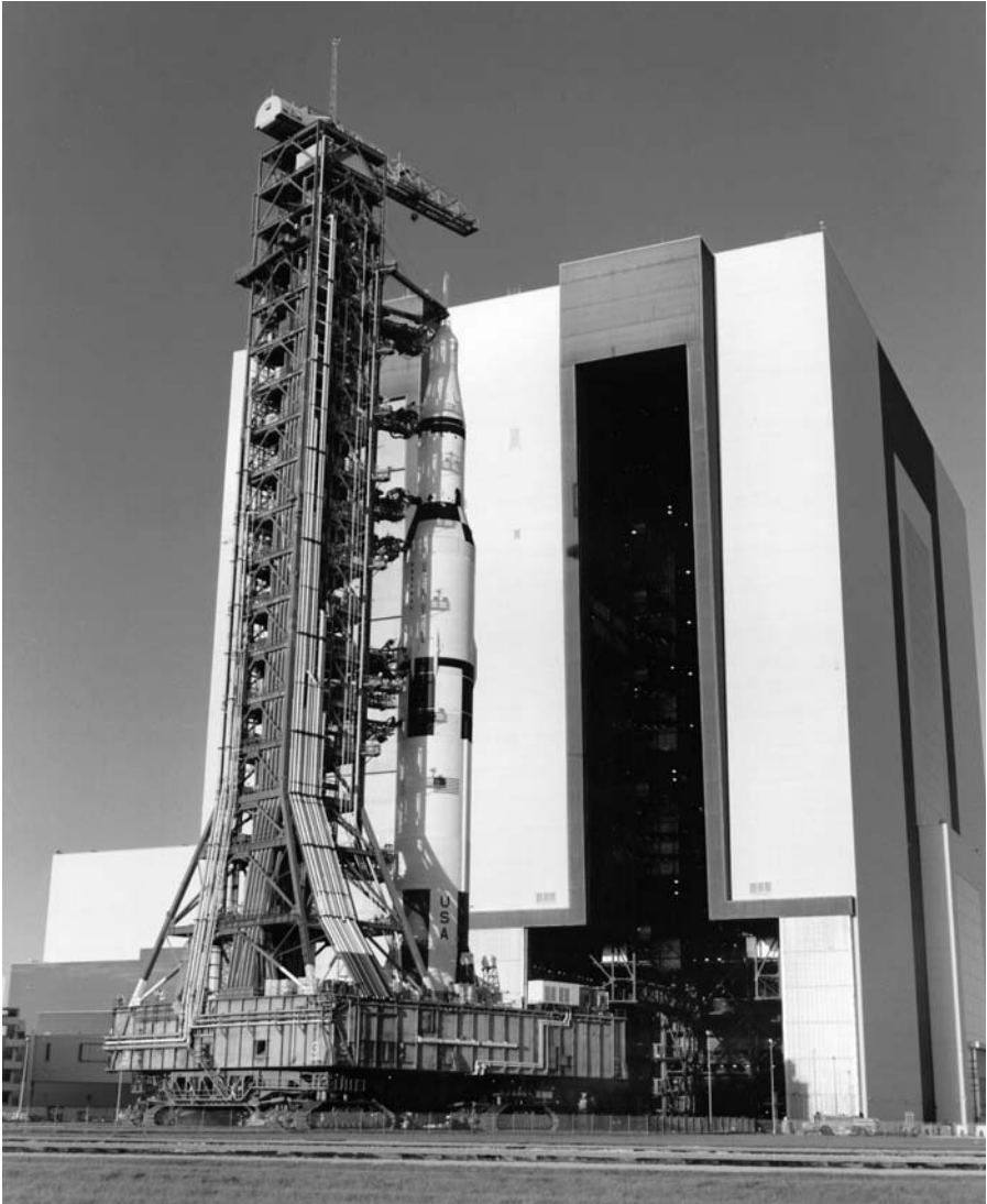
FIGURE 4.1 Apollo 17 Saturn V launch system and spacecraft during transport to its launch pad on the Mobile Launcher Tower. The Vehicle Assembly Building stands behind. The Saturn V booster and spacecraft combination stands 364 feet tall. (NASA Photograph KSC-72PC-426HR)
