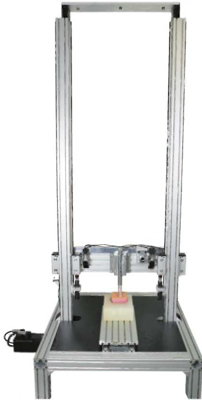
Fig. 11.6 Drop testing setup for analyzing soft-tissue injury during blunt and sharp contact
