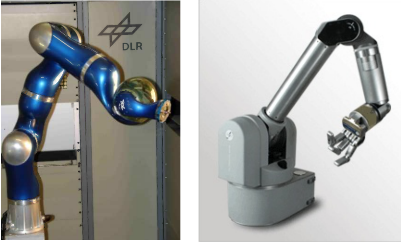
Fig. 2.3 The DLR Lightweight Robot III [19] (left) and the Barrett WAM Arm (right) [62]
