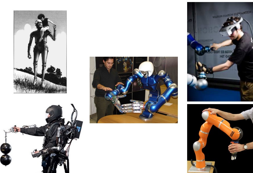
Fig. 1.1 Physical Human-Robot Interaction: The upper left image shows a scene from the robot story Robbie written by Isaac Asimov. In the lower left a human is equipped with an exoskeleton developed by Sarcos Inc. [5]. The center image depicts a human interacting with the DLR humanoid upper body system Justin (middle), the upper right a human attached to a bimanual haptic interface, and the lower right a human interacting with the LWR-III.
