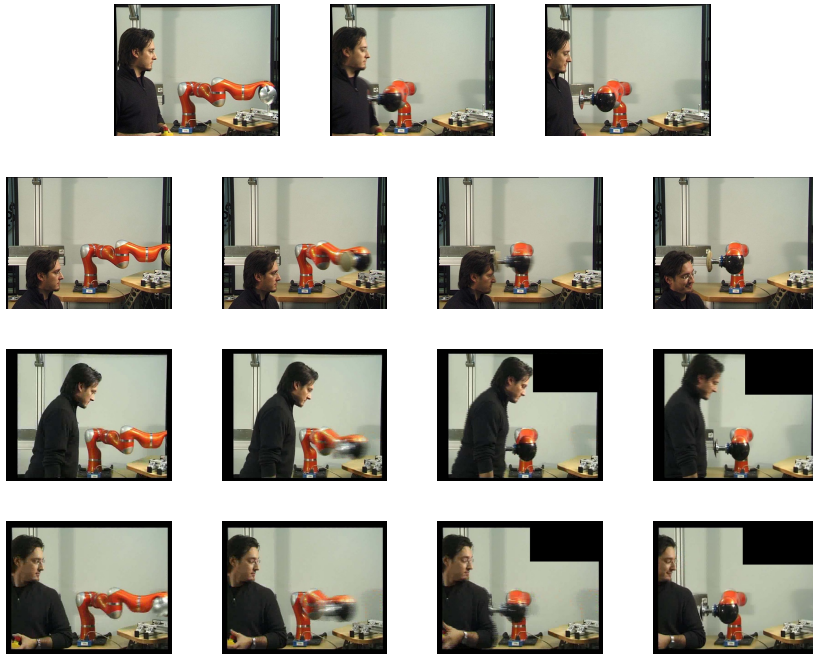
Fig. 5.13 Impact tests with a human chest at 2.7 m/s and head at 1.5 m/s. The impact velocities for the abdomen and the shoulder were 2.7 m/s as well, which is the maximum velocity of the robot. During all these experiments the robot does not react to the activated collision detection. The robot stopped only due to an exceedance of the maximum nominal joint torques. However, as a result from the crash test dummy experiments, the impact forces caused by the very short collision duration cannot be affected by this feature due to its delayed reaction. These test were initially shown in [11] and support, if not even prove the previously given conclusions.
