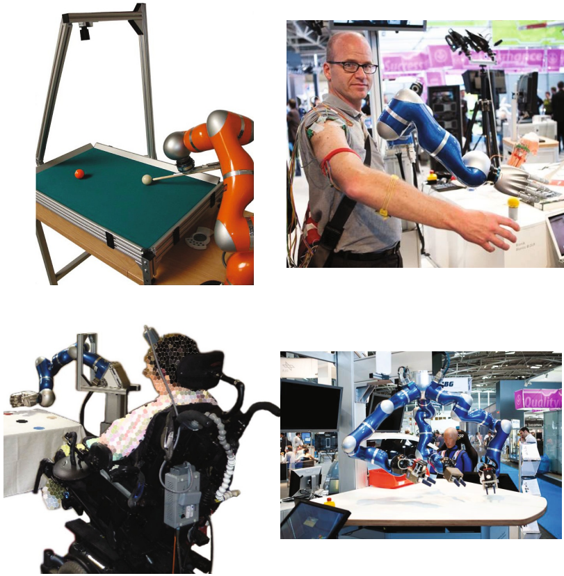
Fig. 12.1 Several example setups using the developed safety oriented state-based robot control architecture. LWR-III controlled via Brain-Machine Interface, SAPHARI setup, Billiard playing and EMG-controlled robot.
