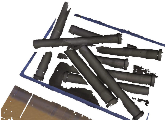
Fig. 8.10 Generated 3D model from a series of sweep scans over the filled bin
