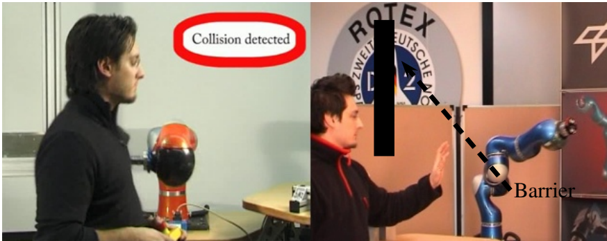
Fig. 3.20 Real collisions with the chest and arm were conducted up to a robot velocity of 2.7 m/s
