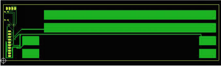
Fig. 3 Top layer containing the electrodes
