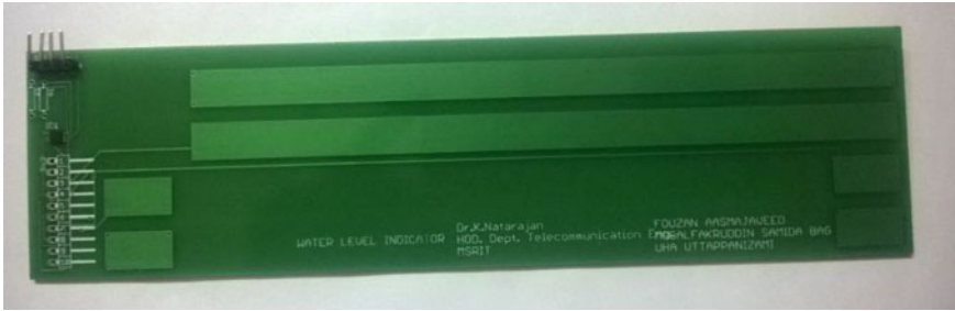
Fig. 6 Fabricated capacitance liquid level sensor
