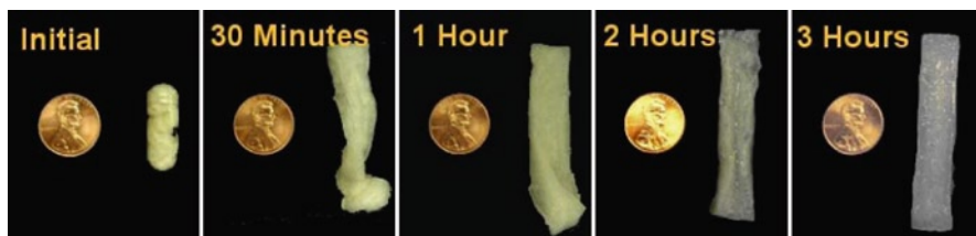
Fig. 17.7 Hydration of the gastric retentive formulation used in Study 1 as a function of time in 0.1 N HCl
