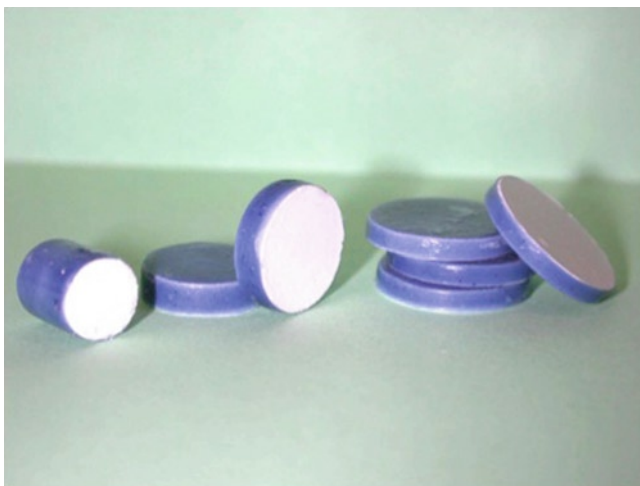
Fig. 11.2 Picture of different sizes of core-in-cup matrices obtained by coating one base and the size surface of the disk
