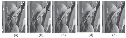
Figure 7. Processing example of output images with different E_b/N_0 (dB) value using raised cosine filter: (a) E_b/N_0 (dB) = 1, (b) E_b/N_0 (dB) = 2, (c) E_b/N_0 (dB) = 3, (d) E_b/N_0 (dB) = 4, and (e) E_b/N_0 (dB) = 5.
