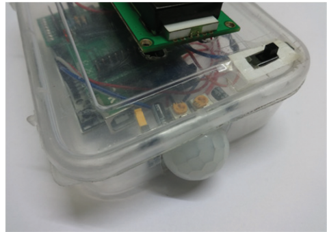
Figure 8. Hardware of end point.
