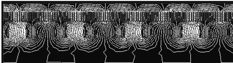
Fig.5. Isopotential line with the consideration of strands insulation and turns insulation when the terminal voltage fluctuate +10%
