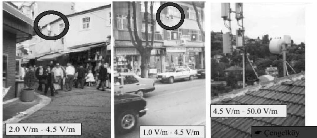
Fig.3. Maximum and minimum measured values for some base stations in Istanbul.
