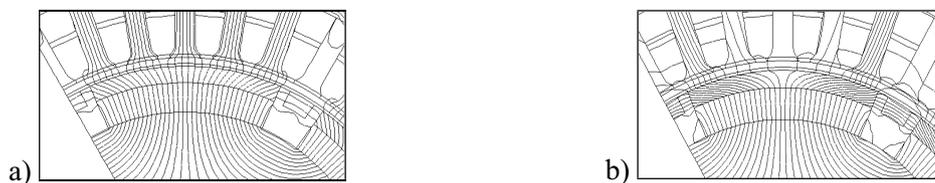
Fig. 6. Rotor 2 under no load conditions (a) and with field weakening current (b)
