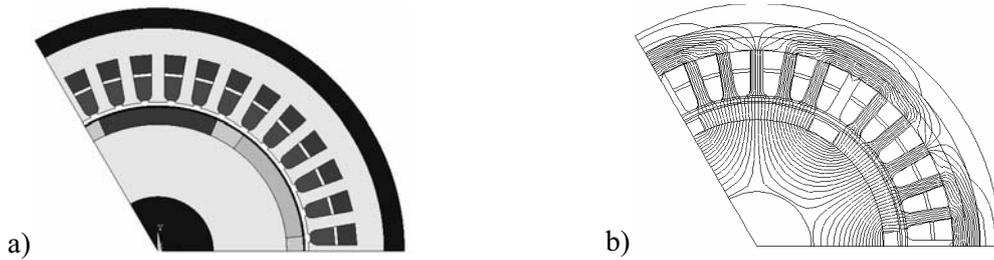
Fig. 3. 120°-section of a 6-pole surface magnet synchronous machine (a) and calculated flux lines under no-load conditions (b)
