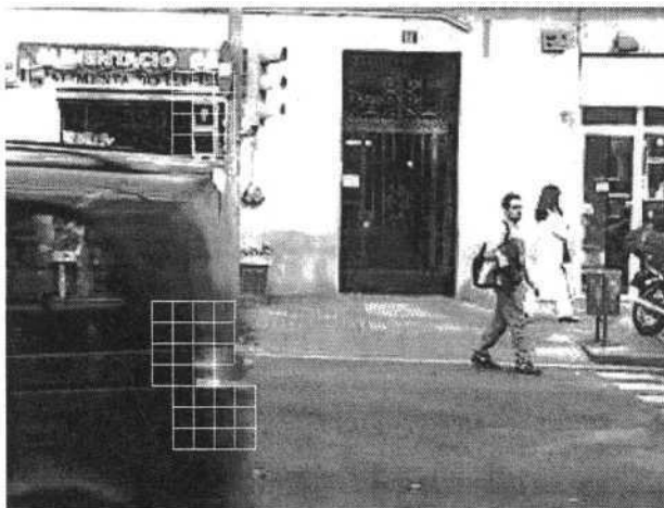
Fig. 2. False candidates in the presence of tail lights of a car.
