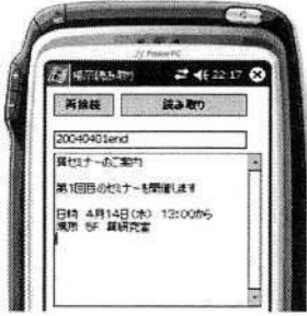
Fig. 4. PDA display after reading a bar code
