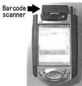
Fig. 2. PDA with a bar code scanner attached to it
