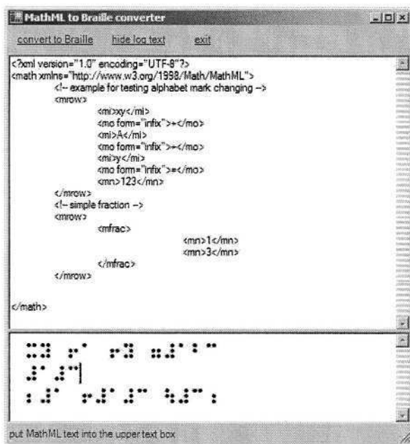
Fig. 1. Screenshot of prototype MathML to Braille converter.
