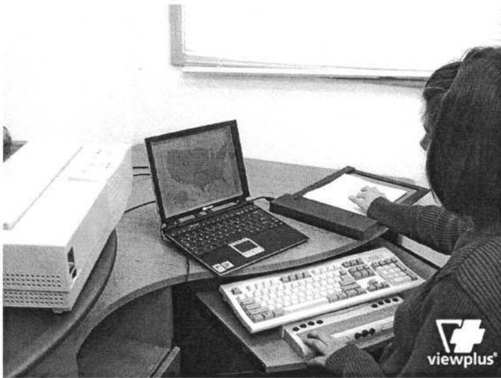
Fig. 1. Photograph of young blind woman examining a US map using the ViewPlus SVG Reader computer application and ViewPlus touch pad. The ViewPlus Cub Tiger tactile graphics and braille embosser is on her left. Any graphic on screen can be embossed on the Cub and placed on the touch pad
