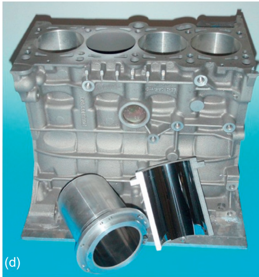
Figure 4.18, cont'd and (d) coated components: four cylinder light-metal crankcases and single light-metal bush.
