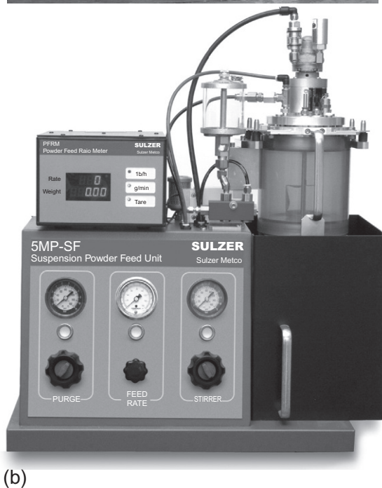
Figure 4.10 Suspension feeder concepts: (a) NanoFeed from Northwest Mettech Corp., Vancouver, Canada; (b) pressurized feeder prototype from Sulzer AG, Wohlen, Switzerland (Cotler et al., 2011).
