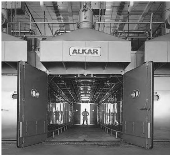
FIGURE 6.1 Large-batch meat processing oven. (From Alkar-RapidPak, Inc. With permission.)
