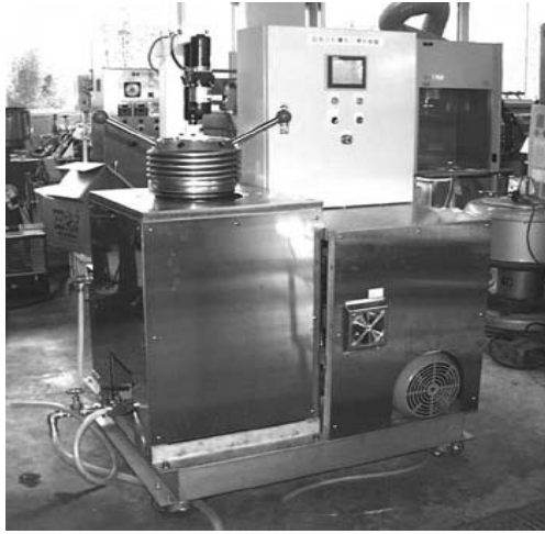
FIGURE 17.22 Photograph of a machine shucking oysters for testing.
