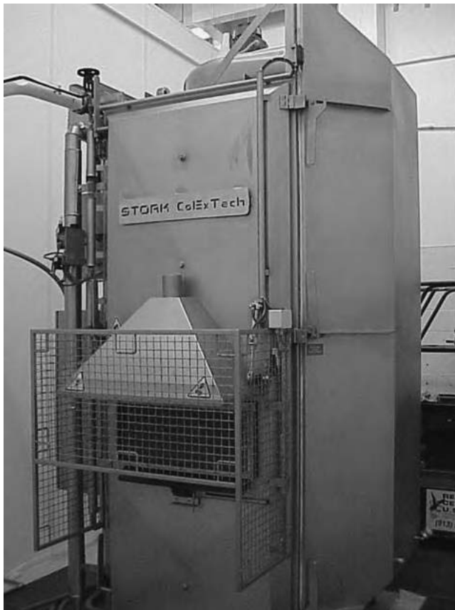
FIGURE 6.10 Townsend condensing steam postprocess surface pasteurization system. (From Townsend Engineering, Des Moines, IA. With permission.)
