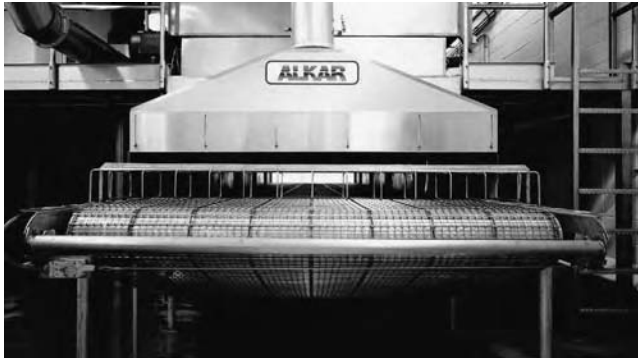
FIGURE 6.5 Air impingement steam cooking system. (From Alkar-RapidPak, Inc. With permission.)
