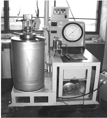
FIGURE 17.3 Photograph of pressure treatment machine for testing the larger volume of samples.
