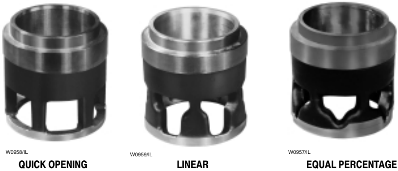
Figure 3-27. Characterized Cages for Globe-Style Valve Bodies
