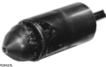
Figure 5-6. Typical Appearance of Flashing Damage
