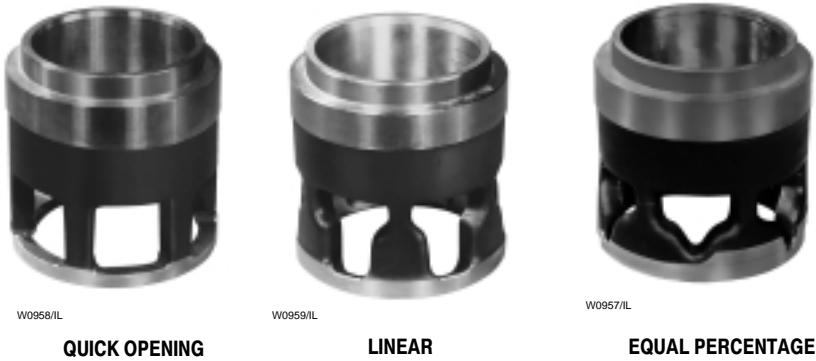
Figure 1-8. Characterized Cages for Globe-Style Valve Bodies
