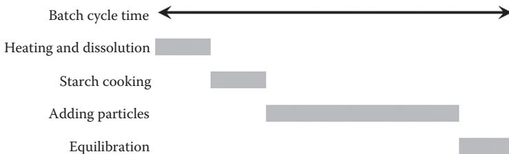
FIGURE 3.5 Typical batch cycle diagram for cook vessel of particulate process.
