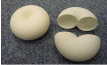
Fig. 7. Model 6: horn torus, constructed by selective laser sintering; d = 2.5 cm, r = 2.5 cm
