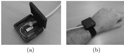
Fig. 2. JoyWarrior 24F8 in housing (a), wrist mounted (b)
