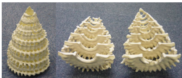
Fig. 1. Radiolarian (Tower type), Scientific name: Svinitzium pseudopuga Dumitrica, Real size: 200 \mu\text{m} , Shape data: Micro X-ray CT, Left (complete model): 24 cm (ratio: 1200 times), constructed using selective laser sintering (nylon powder), Right (partitioned model): 18 cm (ratio: 900 times), constructed by 3D printing (plaster powder)
