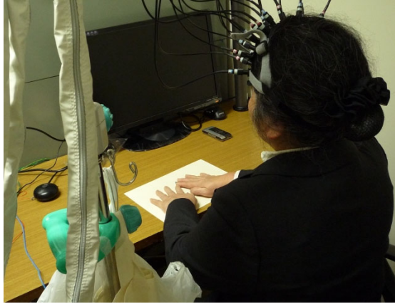
Fig. 1. A subject with NIRS. IR receptors were placed on subject's scalp and their positions correspond to cortical areas.
