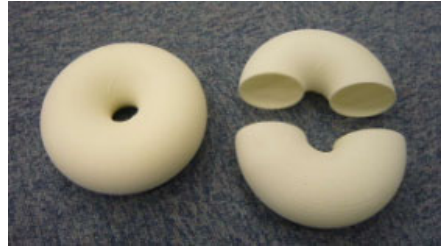
Fig. 6. Model 5: ring torus, constructed by selective laser sintering; d = 5 cm, r = 2.5 cm
