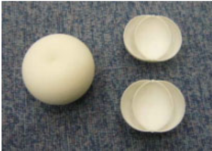
Fig. 9. Model 8: spindle torus, constructed by selective laser sintering; d = 0.625 cm, r = 2.5 cm
