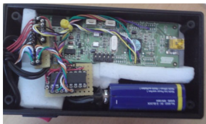
Fig. 2. Experimental version of the electronics box: microcontroller board, programmable gain amplifiers, and power supply with a 9V battery
