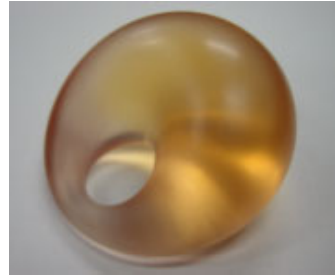
Fig. 2. Model 1: Dupin cyclide constructed by stereolithography; width = 7 cm
