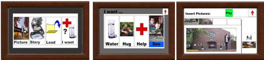
Fig. 2. Final prototype: main menu (left), need tool (middle), the story tool (right)
