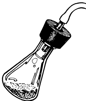
FIG. 1 Drying N-acetyl-DL-alanine under reduced pressure.
