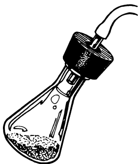
FIG. 5 Drying a solid by reduced air pressure.
