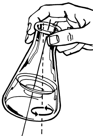
FIG. 1 Swirling of a solution to mix contents and help dissolve material to be crystallized.
