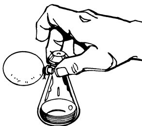
FIG. 1 Apparatus for Brown hydrogenation.
