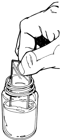
FIG. 3 Preparation of TLC plates by dipping. The two microscope slides are grasped at one end, dipped into the silica gel slurry, removed and separated, and dried and activated by heating.
