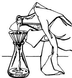
FIG. 2 Gravity filtration of hot solution through fluted filter paper.
