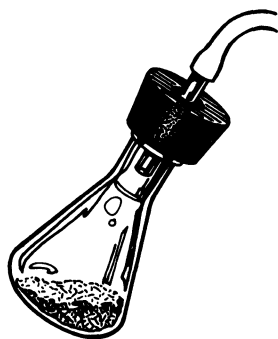
FIG. 3 Drying of acetanilide under reduced pressure. Heat flask on steam bath.
