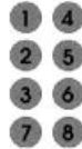
Fig. 1. Each cell is made of 8 dots numbered in the traditional way like represented on this figure
