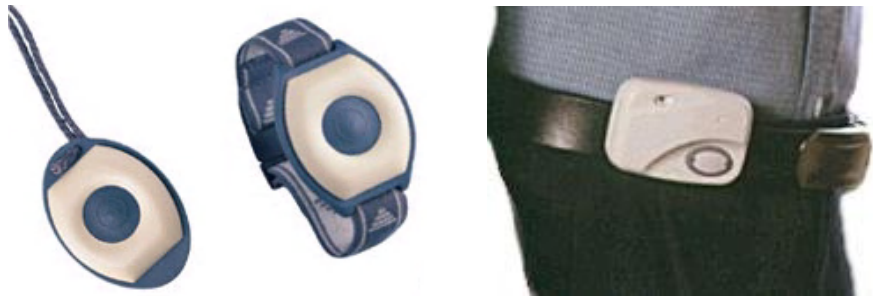
Fig. 1. Left: Examples of wrist or neck worn alarm buttons (Attendo), Source: www.telelarm.de . Right: Fall Detector (Tunstall), Source: www.tunstall.de
