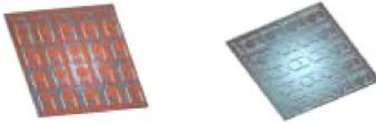
Fig. 1. Model of 5x4 array of micro switches for tactile illusion applications: Bottom View ( left ) and Top View ( Right )
