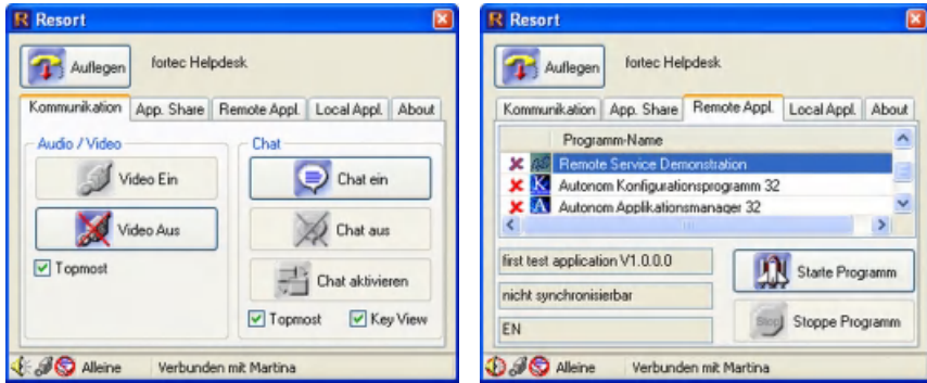
Fig. 3. Screen Shots from RESORT Service Centre during a Tele-Service Session. Left picture shows controls for video and text communication, right picture contains controls for remotely starting and terminating RT applications at the client side
