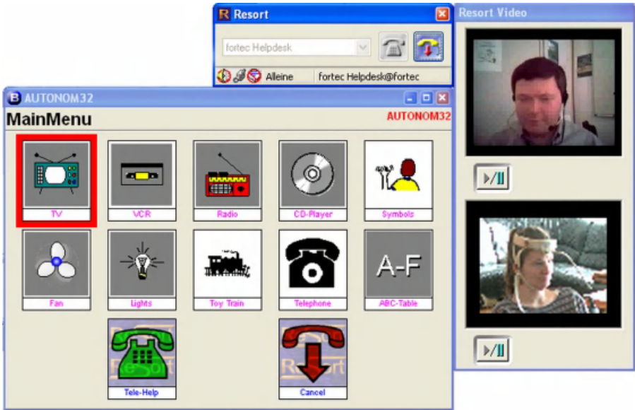
Fig. 2. Screen Shot from a RESORT Client during a Tele-Service session in Vienna. A non-speaking head stick using person runs an environmental control and communication system called AUTONOMY [31], [35] which is equipped with a RESORT Interface. The service centre can be called from inside the AUTONOMY system
