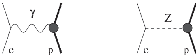
Figure 2.18. Lowest-order Feynman diagrams contributing to electron–nucleon scattering. The electroweak currents of the nucleon are indicated by solid blobs.
