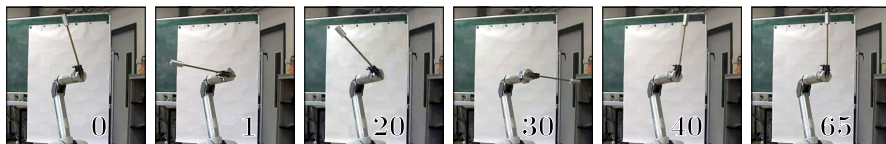
Fig. 4.7 This figure shows the improvement of the policy over rollouts. The snapshots from the video show the final positions. (0) Initial policy after imitation learning (without torque limit). (1) Initial policy after imitation learning (with active torque limit). (20) Policy after 20 rollouts, going further up. (30) Policy after 30 rollouts, going too far. (40) Policy after 40 rollouts, going only a bit too far. (65) Final policy after 65 rollouts.
