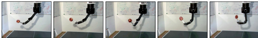
Fig. 3.7 Generalization to various targets (five different forehands at posture ③) are shown approximately when hitting the ball
