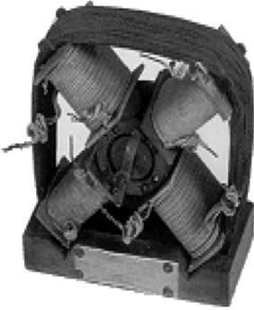
**Figure 1.1** Induction machine at early stage of development.
