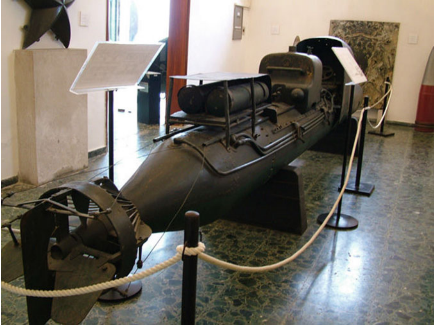
Fig. 1.10 Pig , manned vehicle used by the Royal Italian Navy during the Second World War in the Mediterranean Sea. The thruster and the group rudder/stern can be observed in the bottom left angle of the photo
