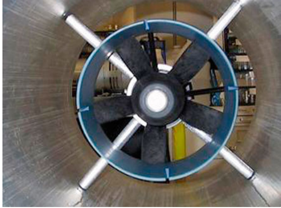
Fig. 2.2 Thruster of SAUVIM (courtesy of J. Yuh, Autonomous Systems Laboratory, University of Hawaii)
