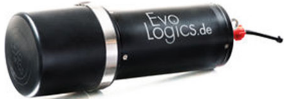
Fig. 1.12 USBL Underwater Acoustic USBL System, device for tracking and communication in shallow waters, providing data transfer rates nomially up to 31.2 kbit/s over a 1,000 m range (courtesy of EvoLogics GmbH)
