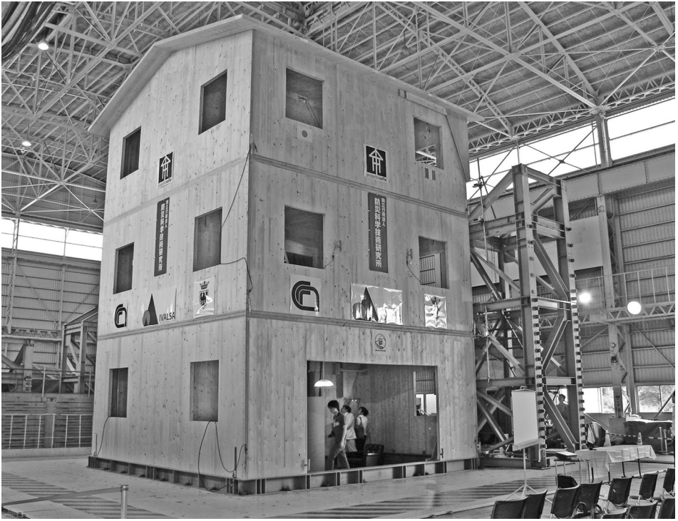
Figure 11.1 Testing a full scale three-storey timber building on the Tsukuba shaking table, Japan (reproduced from Ceccotti et al. , 2007; photograph courtesy of Maurizio Follesa, taken as part of the research project, Progetto Sofie (Sofie Project), funded by the Province of Trento, Italy, and carried out through CNR-IVALSA (Trees and Timber Institute), Italy)
