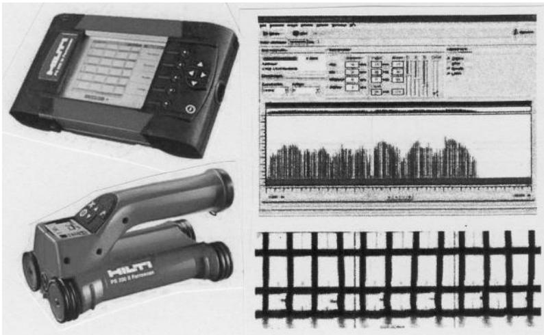
Figure 6.12 Control of achieved concrete cover based on scanning systems. (From Grantham, M., *The Use of NDT Methods in the Evaluation of Structures*, in *Proceedings, Second International Symposium on Service Life Design for Infrastructure*, vol. 2, RILEM, Bagnex, France, 2010, pp. 1003–1012.)
