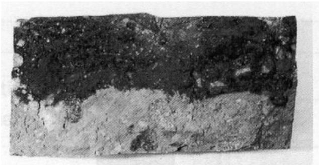
Figure 6.5 Observed depth of chloride penetration on the split concrete surface after spraying of the fresh surface with a standard  $\text{AgNO}_3$  solution.
