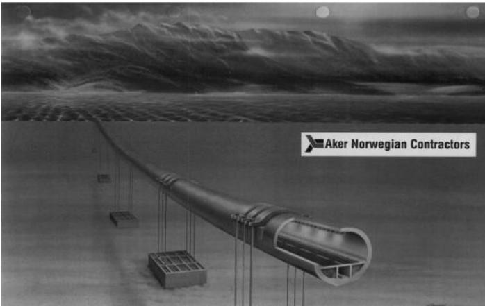
Figure 1.7 One of several designs studied for possible strait crossings by use of submerged tunnels. (Courtesy of the Norwegian Public Roads Administration.)
