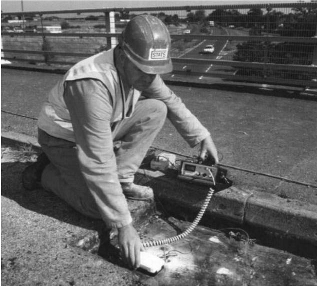
Figure 6.11 Control of achieved concrete cover based on the pulse induction technique. (From Germann, *In-Situ Test Systems for Durability, Inspection, and Repair of Reinforced Concrete Structures*, Germann Instruments A/S, Copenhagen, Denmark, 2008, <http://www.germann.org/>.)
