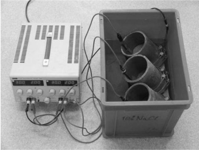
Figure 6.4 Concrete specimens under testing with the RCM method. (From NORDTEST, *NT Build 492 Concrete, Mortar, and Cement Based Repair Materials: Chloride Migration Coefficient from Non-Steady State Migration Experiments*, NORDTEST, Espoo, Finland, 1999; Tang, *The RCM Test (NT Build 492) for Evaluating the Resistance of Concrete to Chloride Ingress*, Tang's CI Tech, Gothenburg, Sweden, 2008, tang.luping@bredband.net.)
