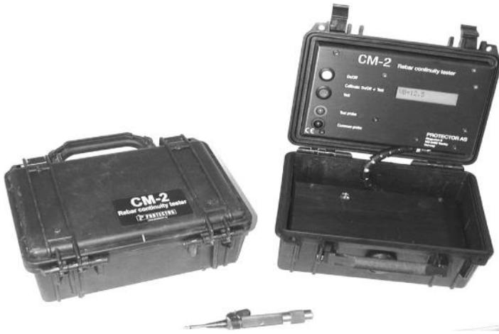
Figure 6.13 Equipment for control of electrical continuity within the reinforcement system. (From Protector, CM2 Rebar Continuity Tester, Protector AS, Oslo, Norway, 2008, [http:// www.protector.no/](http://www.protector.no/))
