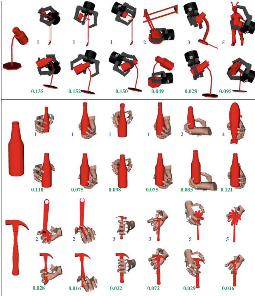
Fig. 11 Three example models and their grasps, using the database-backed planner with Zernike neighbors. For each model \alpha (left), the top row of images shows a neighbor n_k from the database, the value of k , and a pre-computed grasp on that neighbor. Directly below each neighbor is the same grasp executed on \alpha , along with its GWS epsilon quality measure
