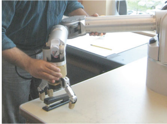
Fig. 1 The physical human interactive grasping environment: the human physically guides the robot wrist and fingers into a grasping posture
