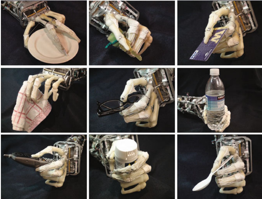
Fig. 11 The ACT Hand can grasp everyday objects with human-like finger postures. Figures show grasping of nine objects, namely, a coffee plate, key, credit card, hand towel, glasses, water bottle, cordless phone, medicine bottle, and spoon, which are identified as important for ALS patients [9]
