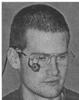
Fig. 1. Location of the camera in the MEMREC system
