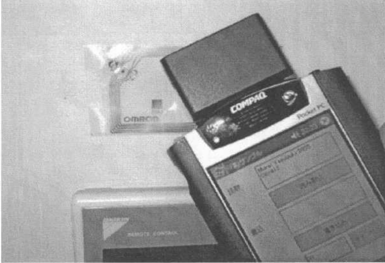
Fig. 8. Reading an RFID tag by reader-writer attached to PDA
