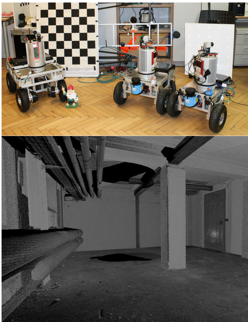
Fig. 1 Left: The robots we used in our calibration experiments. From left to right: Achim3D, Lars3D and Irma3D. The red/silver cylinder on top of the robots is the Riegl VZ-400 laser scanner. Right: The geodetically measured model of the basement (colored by reflectance).
