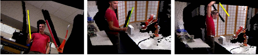
Fig. 3 Screen shots showing the precision and robustness of the RANSAC segmentation [8] of the human’s sword (yellow) in different configurations
