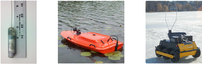
Fig. 1 Our robotic system consists of radio tags, a radio antenna and receiver mounted on autonomous boat in summer and wheeled rover in winter (to operate on frozen lakes)
