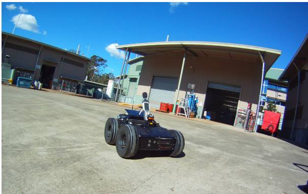
Fig. 2 The robot used in the experimental campaign showing the sound pressure level meter, Hokuyo laser scanner and computing hardware
