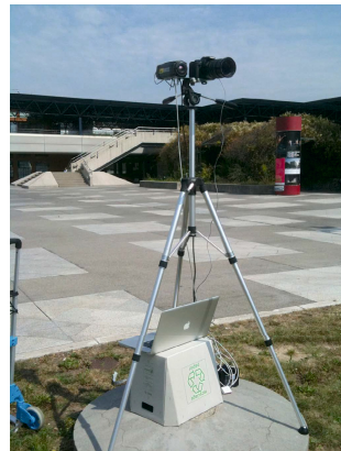
Fig. 2 The camera rig consisting of a thermographic camera and a digital true-color camera mounted on a pan-tilt head
