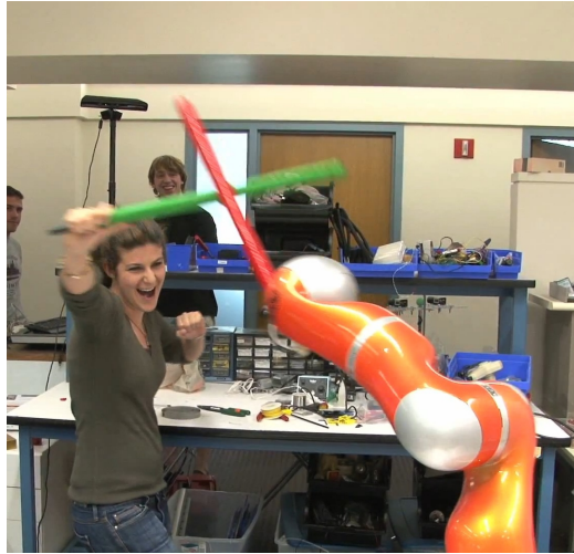
Fig. 1 Reactive motion generation and control during physical human-robot interaction with “JediBot”
