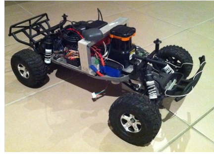
Fig. 1 The rOscar platform is a 1/8th scale RC car platform. It is equipped with a Hokoyu UTM-30LX laser scanner, a Microstrain 3DM-GX2 IMU, odometry and current sensors. The onboard processor is a Gumstix Overo running ROS and running drivers as published in the cyphy ROS repository. See [9] for more details.
