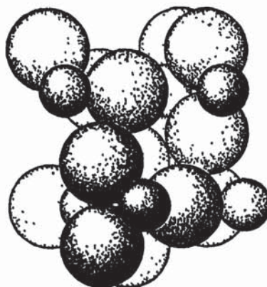
FIG. 289a.—(left) The improved structure for \text{Fe}_3\text{C} projected on the b -face of its orthorhombic cell. The large circles are the iron atoms.
