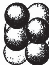
FIG. 275a —(left) The unit cell of the new orthorhombic arrangement found for metallic gallium as projected on its b-face.
