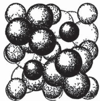
FIG. 326b.—A packing drawing of a . Si atoms cannot be seen; the Ca ions are line-shaded.
