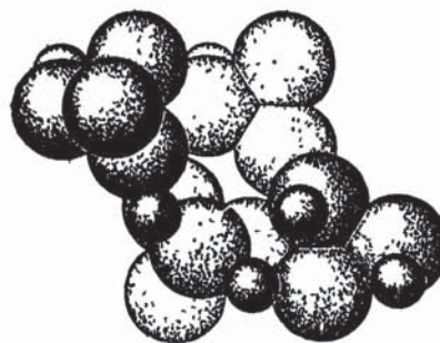
FIG. 311a.—(left) The monoclinic structure determined for \text{Li}_2\text{SO}_4 projected on its b -face. The largest circles are O, the smallest are Li atoms.
