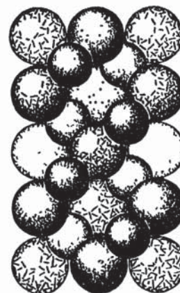
FIG. 293a.—(left) The new arrangement found for chalcopyrite, \text{CuFeS}_2 , as projected upon an a -face. Cu atoms are at the origin; intermediate circles are the Fe and the smallest circles the S atoms.
