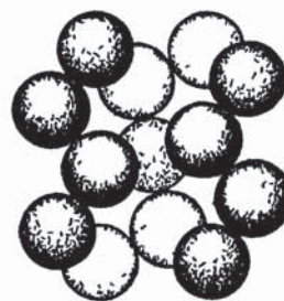
FIG. 278a.—(left) The new atomic arrangement deduced for marcasite, FeS_2 , as projected upon the a -face of its orthorhombic cell. The small circles are Fe atoms.
