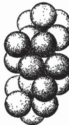
FIG. 313a.—( left ) A portion of the diaspore, \text{Al}_2\text{O}_3 \cdot \text{H}_2\text{O} , structure projected on an a -face. Small circles are Al atoms. Water molecules, as such, do not exist in this grouping.
