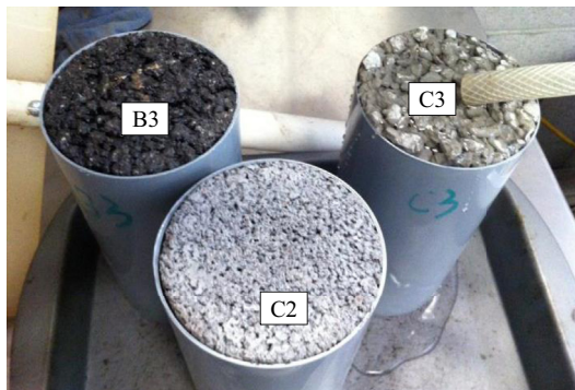
Figure 7.3 Adding water to fill up the cylinder containers.
