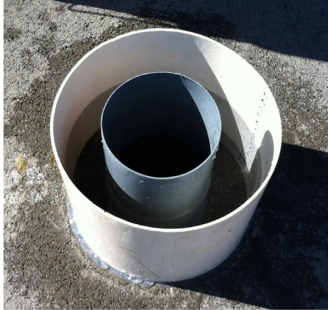
Figure 5.7 Double ring used for testing (compared to the single ring as shown in Figure 5.2 ).
