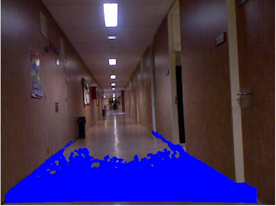
Fig. 4. Example of floor points projected as pixels
