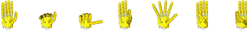
Fig. 3. The seven hand poses used for the calibration sequence, as visualized by the Shadow hand model in GraspIt!. The set includes stretched and fully flexed fingers, finger abduction, and selected thumb poses. The last pose is used to calibrate the palm-arch sensor and the extreme range of the thumb.
