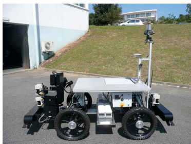
Fig. 3. Robucar-TT platform equipped with IMU, odometry, three range-finder sensors and GPS receiver
