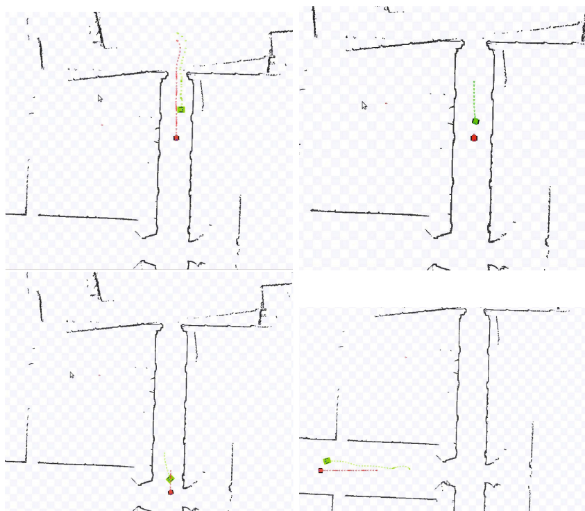
Fig. 6. Typical execution of the POMDP controller guiding the person (green) towards the destination
