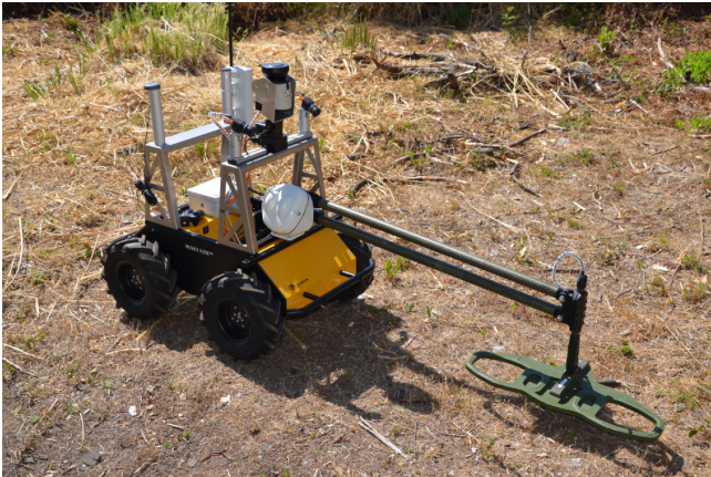
Fig. 1. Robot equipped with mine detecting sensors
