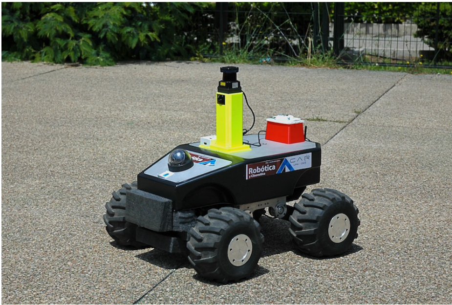
Fig. 2. The complete Summit XL robotic platform. The on-board computer and IMU are inside the chassis. The long range Hokuyo laser and the FireFly camera are mounted on a pedestal to facilitate the detection of the external objects. The shorter range laser rangefinder is below the robot and allows avoiding lower obstacles.
