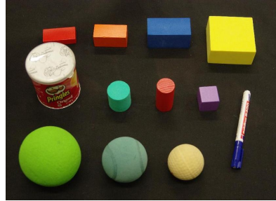
Fig. 4. Attributes of the prototype objects from the IST object set used for the recordings. The objects include three basic shapes (sphere, cylinder, box), different object diameters matched to typical human grasping tasks, and also different materials (wood, metal, rubber, sponge). Values in bold indicate the object dimensions along which opposition forces are applied. Dimensions are in millimeters.
