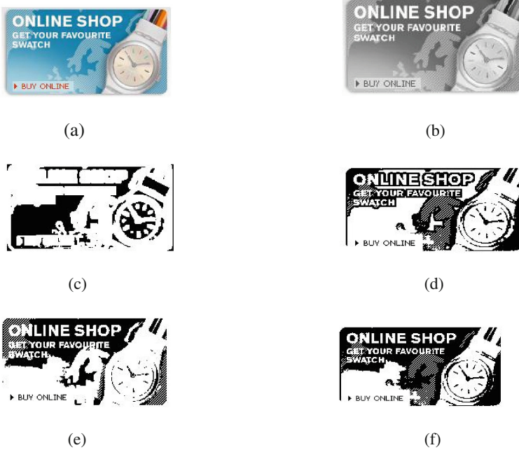
Fig. 3. Steps of Binarization: (a) Input image. (b) Gray scale image of (a). (c) After binarizing variance matrix. (d) After binarizing white region of (c). (e) After binarizing black region of (c). (f) Final binarized image.
