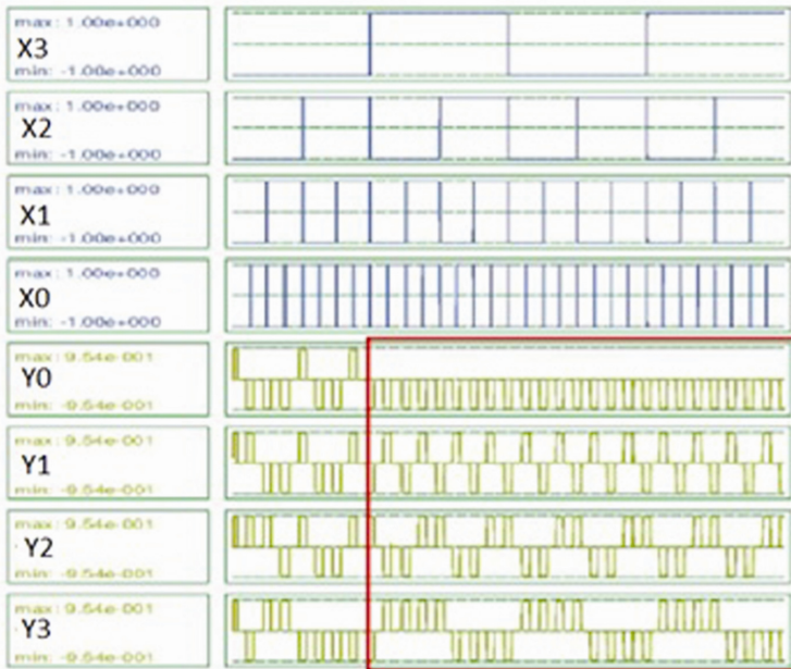
Fig. 13. QCA simulation result of a multiple left shifter for case 2
