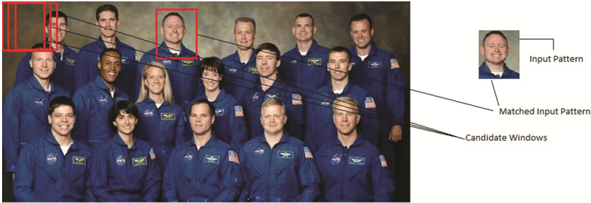
Fig. 1. An Example of Pattern Matching Technique where Input Pattern is compared with all the Candidate Windows and later, best match Candidate Window is determined.
