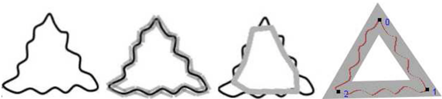
Fig. 2. a. Object b. & c. traditional polygonal approximation d. proposed scheme
