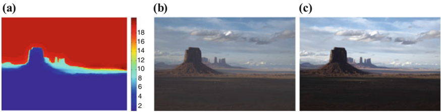
Fig. 6.18 Comparison with the physical model used in [17]. The input photograph and reference are those used in Fig. 6.2. a Estimated depth. b Result by [17]. c Result by the proposed method with the parameter q_C = 0 . The mean saturation is preserved to the original one to make the result comparable with that in b
