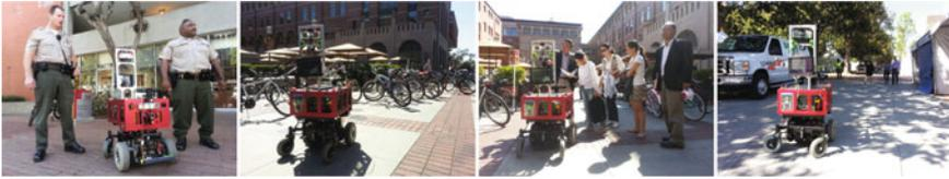
**Fig. 1** Examples of tasks for service robots. From *left to right* patrolling alongside law enforcement personnel, searching for target objects, providing information to visitors, and assessing situations and conditions of the area of responsibility
