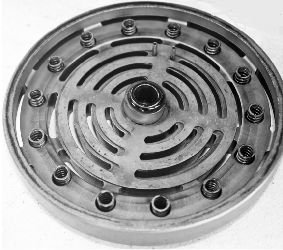
FIGURE 14.6 Valve guard with springs and damper plate.
