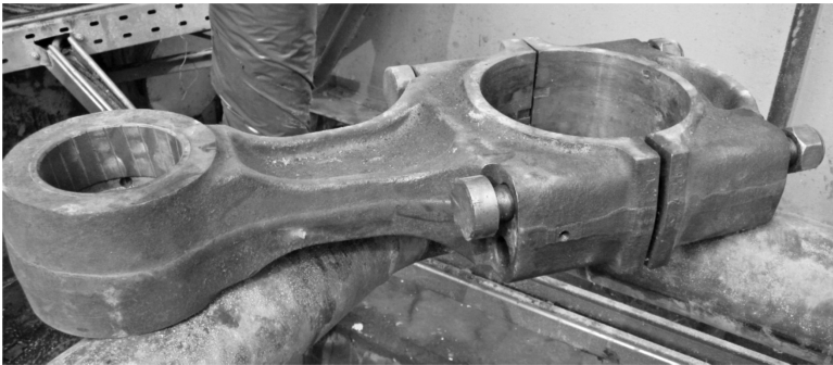
FIGURE 12.8 Connecting rod—moderate speed compressor. (Source: Field photo CES—Superior.)
