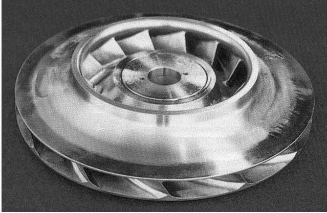
FIGURE 7.1 Typical closed compressor impeller. (Source: Mitsubishi Heavy Industries.)
