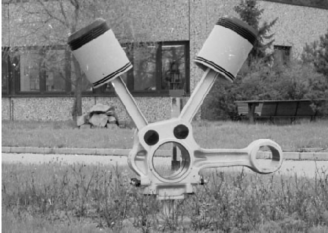
FIGURE 12.9 Connecting rod and articulating power piston rods of an integral gas engine compressor. (Source: Open Grid Europe formerly EON formerly Ruhrgas AG, Germany, NG pipeline compressor station display.)
