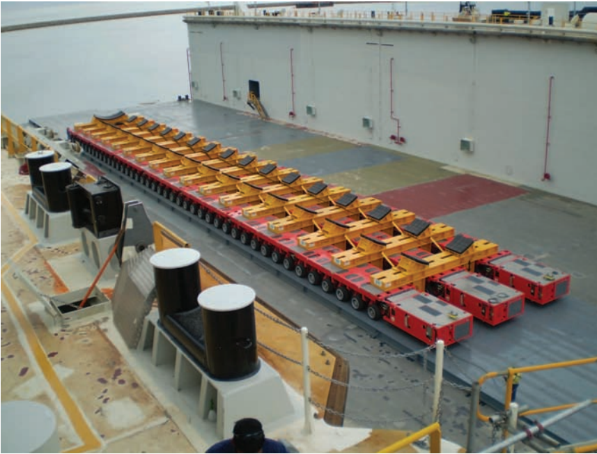
Fig. 10-42. SPMT transfer arrangement
