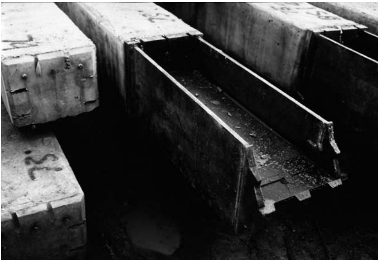
Fig. 8-19. Steel H-pile “stinger” attached to prestressed concrete pile for hard driving conditions
