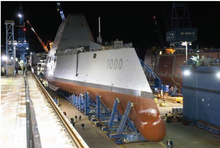
Fig. 10-41. Land level transfer operation onto a floating dry dock launch platform
