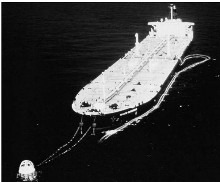
Fig. 9-6. VLCC discharging crude oil at one of three SALM buoys at the Louisiana Offshore Oil Port (LOOP)
