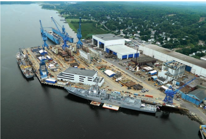
Fig. 1-8. Bath Iron Works LLTF shipbuilding facility providing land-level transfer access to a floating dry dock from three separate building ways
