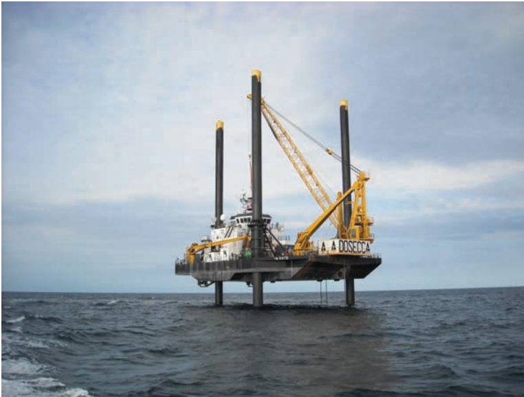
Fig. 8-1. Jack-up barge for deep or rough water drilling
