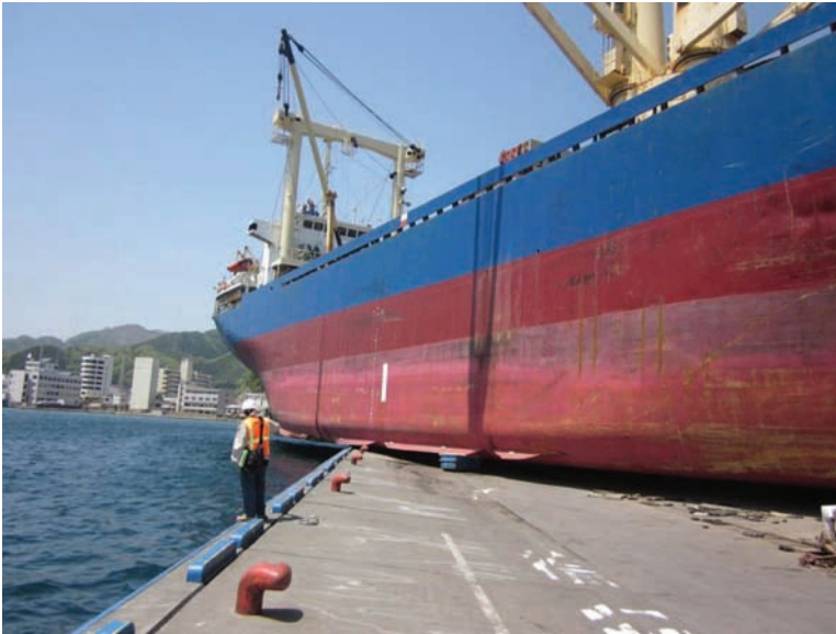
Fig. 4-20. Vessel of 6,175 DWT “beached” on deck of filled wharf at Kamaishi Port, Suga, Japan, because of the Great Tohoku Tsunami of 2011
