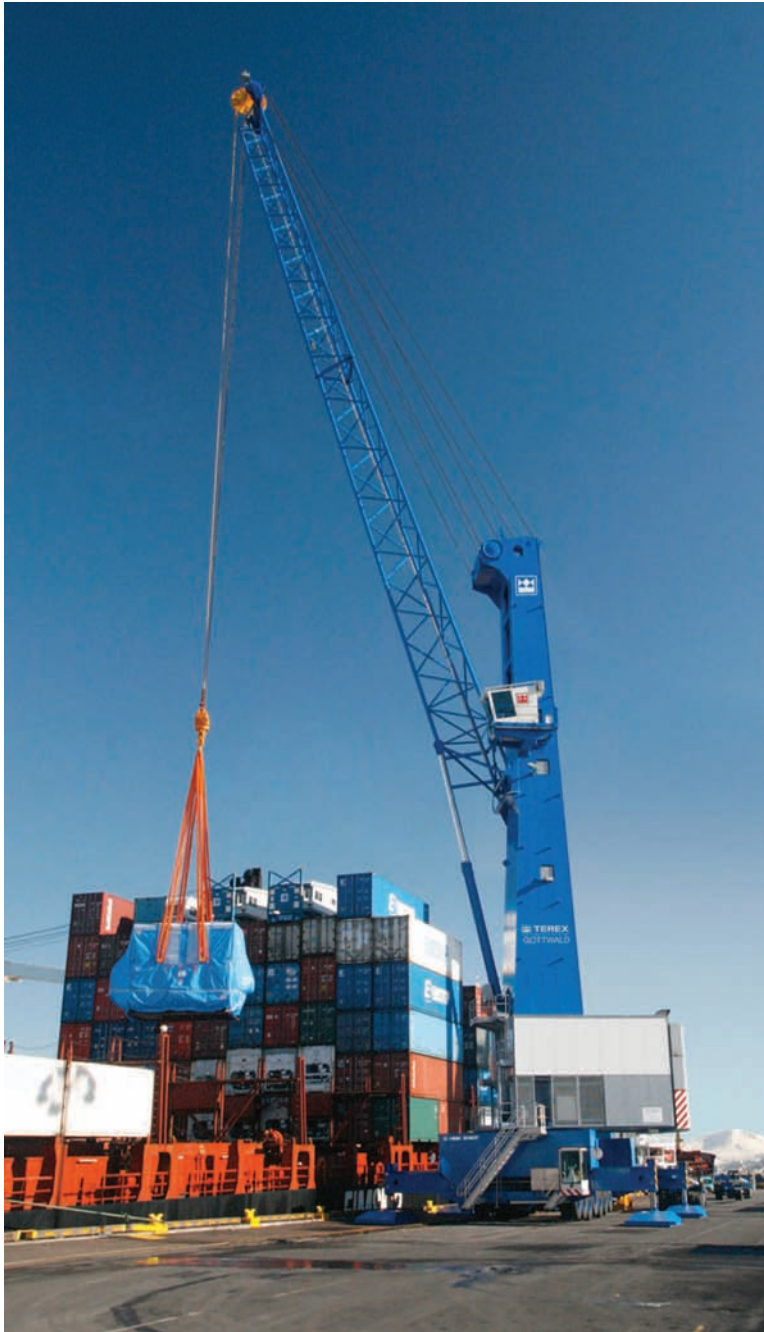
Fig. 4-5. Mobile harbor crane handling containership cargo. This crane has a capacity of 125 metric tons at 20 m reach and has seven axles with 28 wheels
