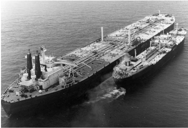
Fig. 2-5. Two tankers engaged in lightering illustrate the dramatic increase in tanker sizes from WW II vintage T-2 to contemporary VLCC
