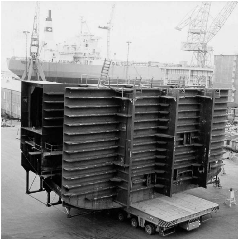
Fig. 4-3. Heavy load transporter in use at ship building yard
