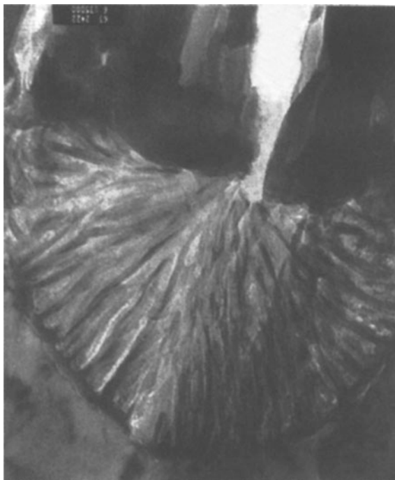
Fig. 1.4 Cross-sectional image of the arc cubic interface on the bottom of an Al oxide layer
