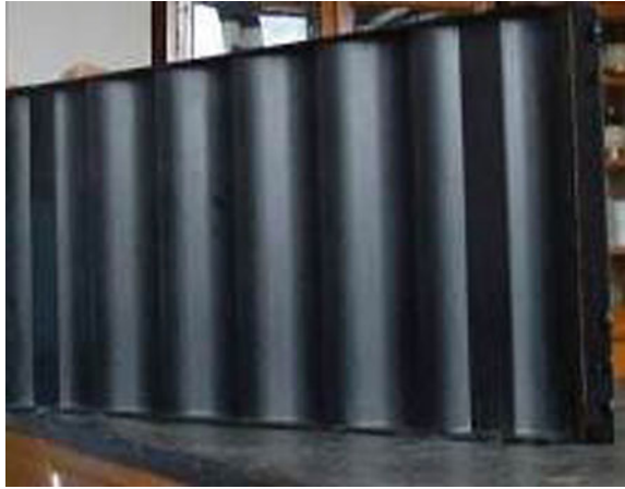
Fig. 1.36 Representative sine-wave beam formed by liquid molding at BIAM
