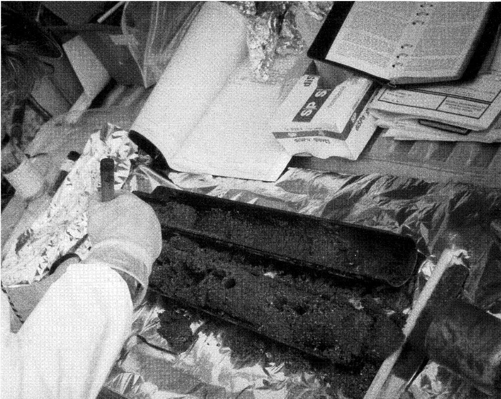
FIGURE 8.22 Hydrogeologist describing a split-spoon sample.
