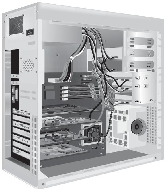
On a desktop PC, the motherboard contains several slots, into which you can plug additional *boards* (also called *cards*) that perform specific functions. Notebook PC motherboards can't accept additional boards and thus aren't expandable like desktop PCs are.
