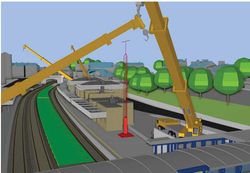
The Cab Secure Radio Mast would have hindered crane movements
