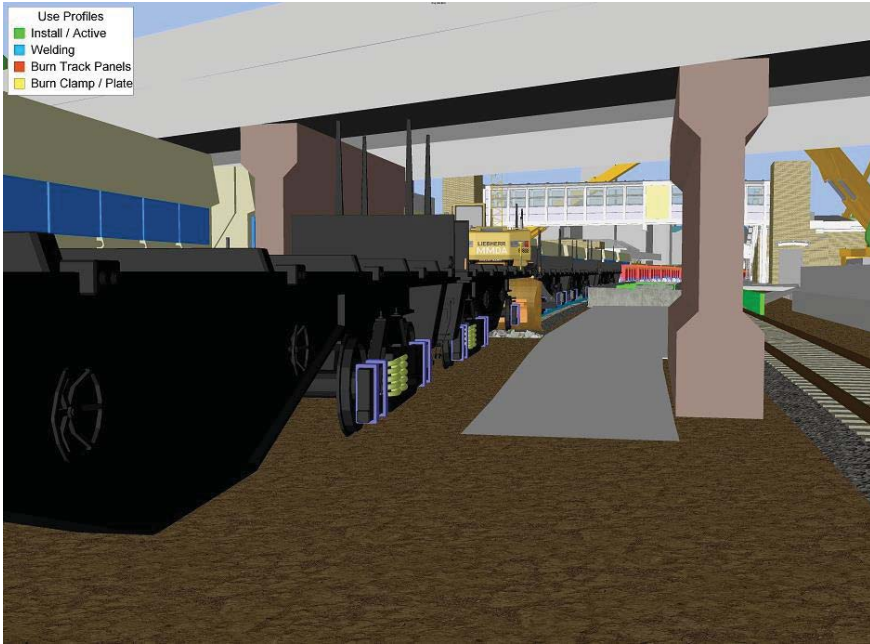
4. An engineering train to be positioned on incomplete track.
