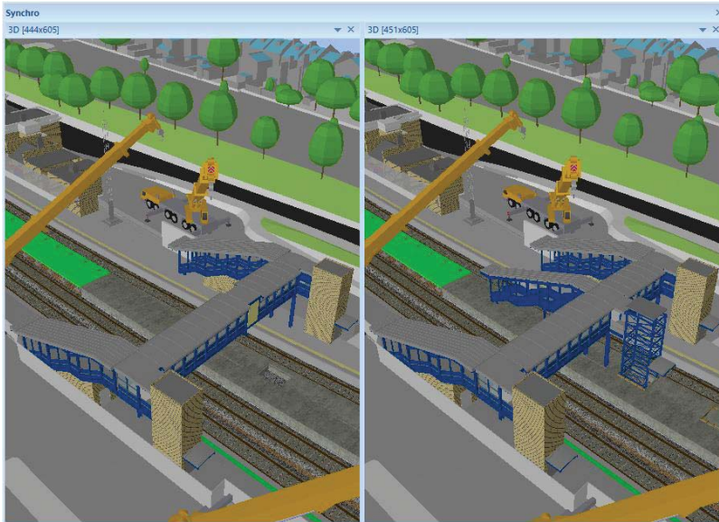
Planned v Actual – Steelwork to central platform delivered 36 hours early
